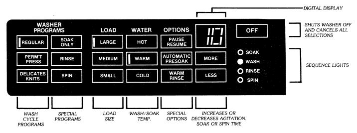
The left portion of the computer touch control panel programs the washer. The washer selections can be seen at a glance. Red indicators light up in the pads of the programmed selections.
